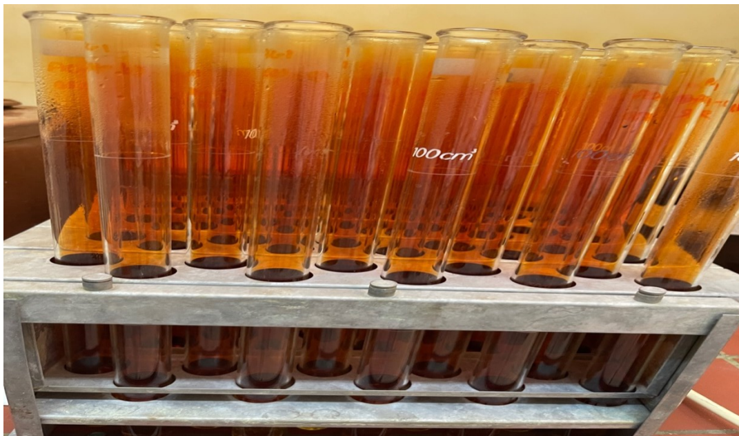
Figure 20 Samples after pre-digestion with Nitric acid
