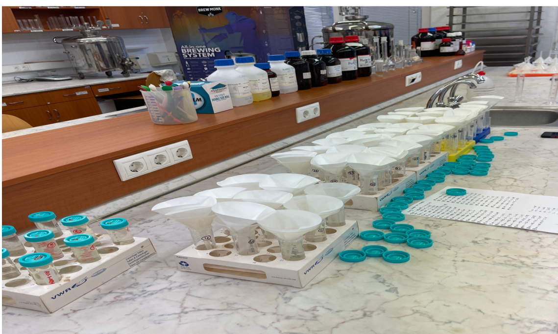
Figure 22 Filtration of digested samples into centrifuge tubes
