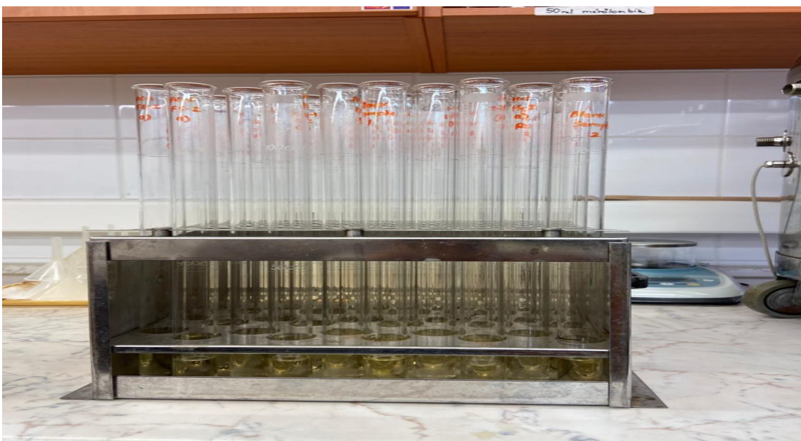
Figure 21 Samples after final digestion with Hydrogen Peroxide
