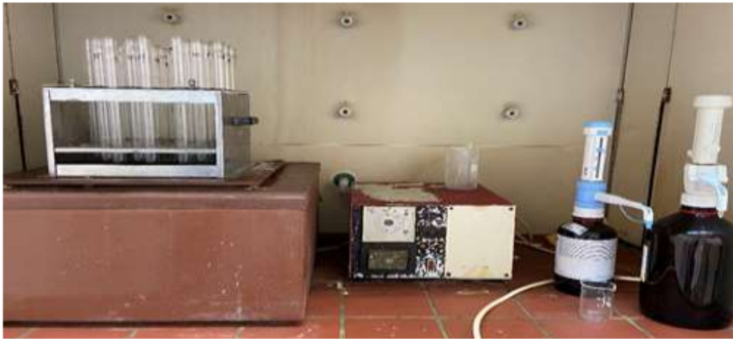
Figure 19 Digestion unit with Nitric acid and Hydrogen peroxide
