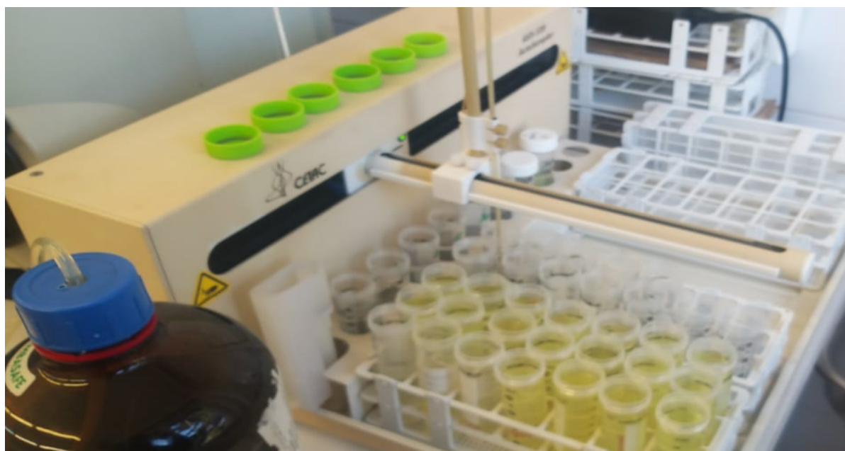
Figure 26 Samples injected through ICP-MS
