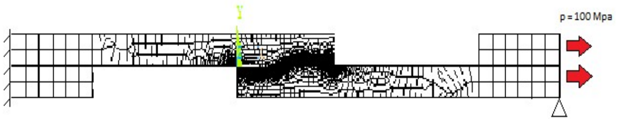
Fig. 2.3. Mesh pattern and boundary conditions
