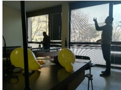
Figure 3:11 Balloon burst for reverberation time measurement in M6
