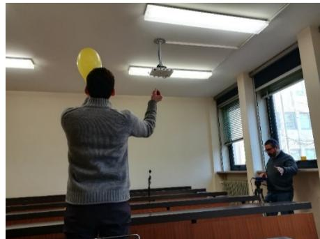
Figure 3:5 Balloon burst for measurement of reverberation time in M5
