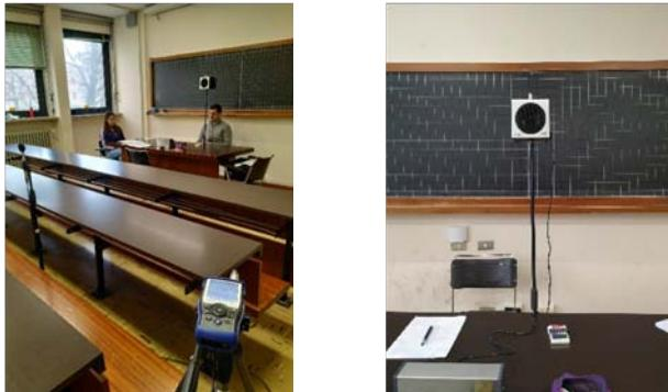
*Figure 3:4 STIPA measurements*
