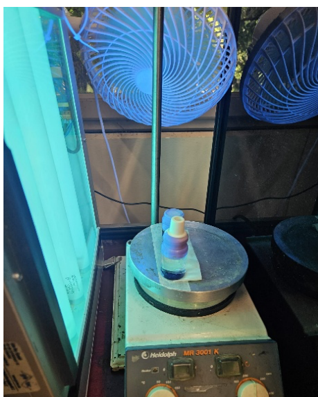
Figure S1: Photo of the polymerization set up. At the side, a fan is present to control the temperature.
