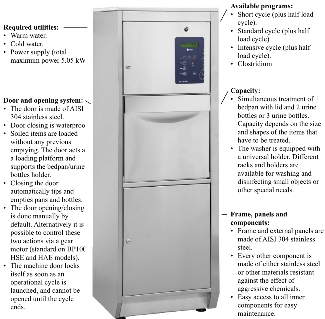
Figure 5.1: BP 100 HE 1000 and some of its features
