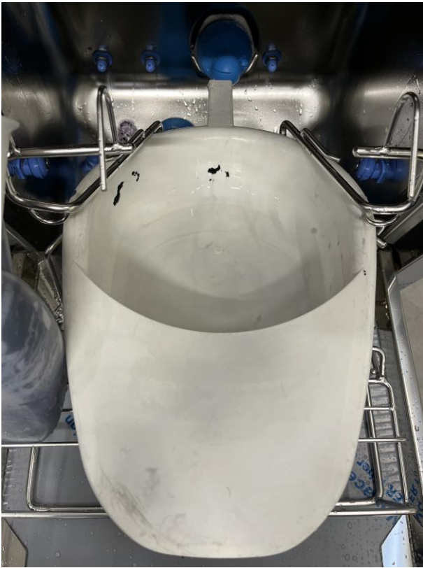
Figure 3. Cleaning results with standard rotating nozzles.
