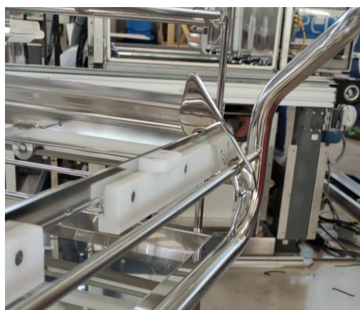
The trolley locking system for the load carrier.
