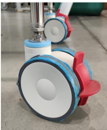
The swivel wheels of the trolley with their lock system.
