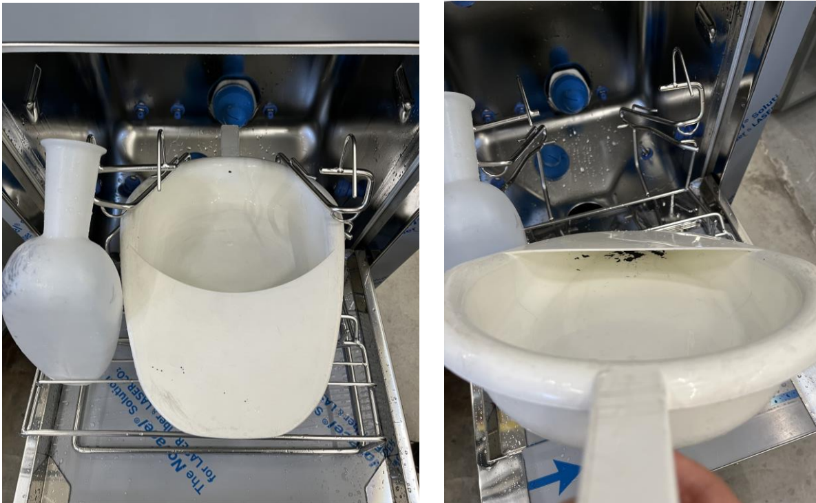
Figure 4. Cleaning results with new rotating nozzles.
