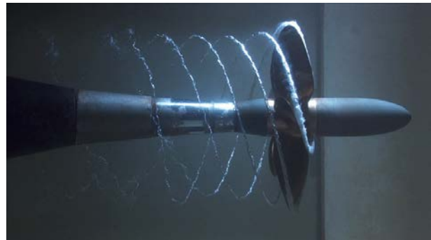
(b) Vortex cavitation. Picture from Bosschers [49]
