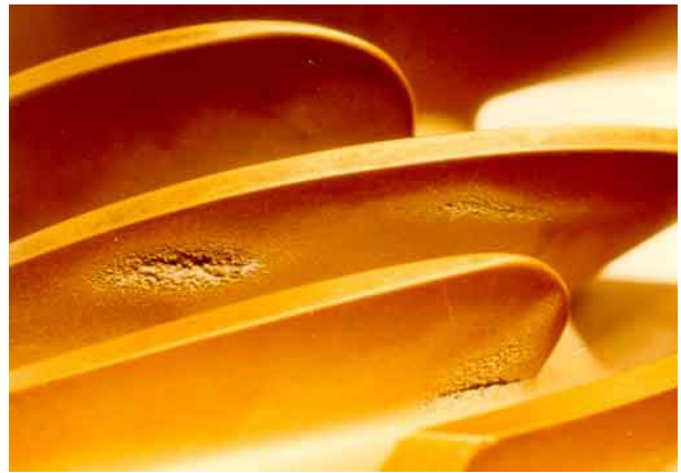
(b) Photograph of typical cavitation damage on the blade of a mixed flow pump. Picture from Brennen [10]
