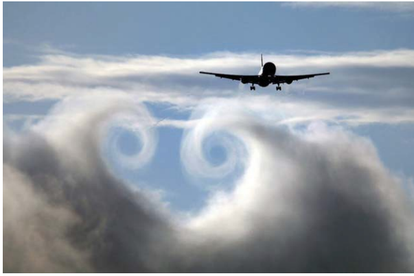
(a) Turbulence phenomena generated in the atmosphere by the wake of a Boeing 767. Picture from Cengel et al. [30]
