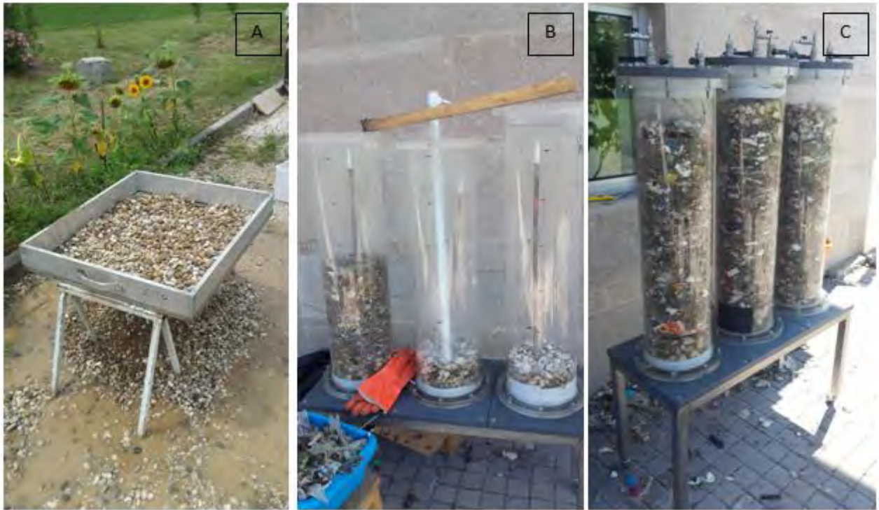
Fig. 9: Filling of the columns. On the left side (A) is shown the “washing station” for the stones. Stones with a diameter of 2cm-4cm before have been placed inside the columns were washed with water. Pictures B and C show the filling phase of the columns.
