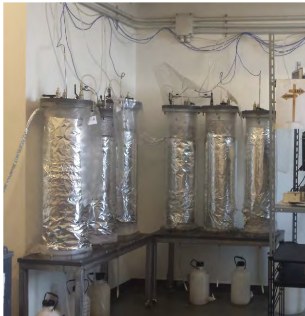
Fig. 4: Final isolation. As last layer was used an aluminum foil.
