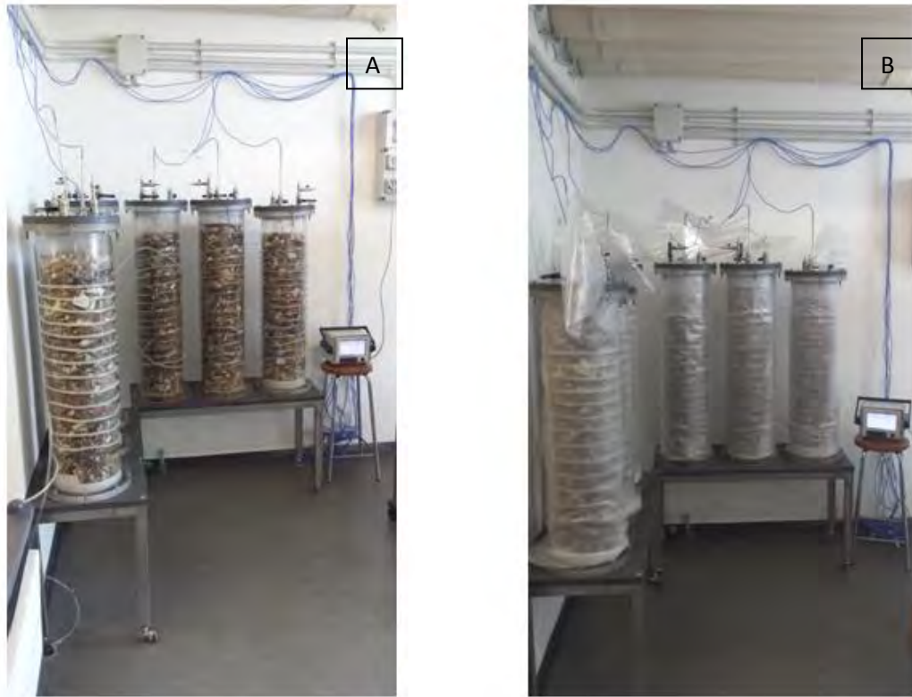
Fig. 3: Steps required for the creation of the insulating system. In the picture A can be seen the PVC pipe wrapped around all the columns. Picture B shows the two layers of pluriball and the picture on the right side the complete “jacket” with the aluminum foil
