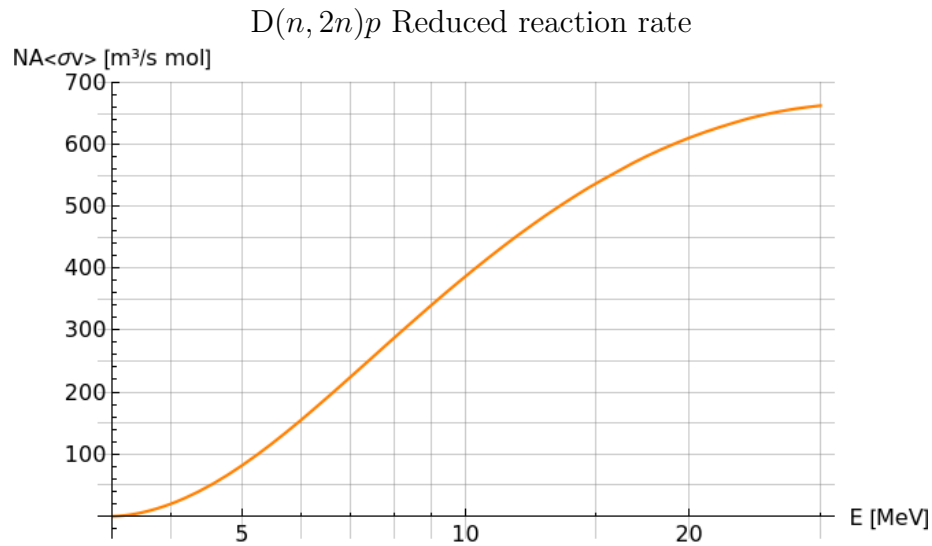
Figure 5.4: Reduced reaction rate N_A \langle \sigma v \rangle for the reaction D(n, 2n)p using the expression 2.2
