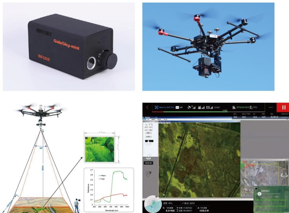
Figura 2.5: Gaiasky-mini Hyperspectral Imaging system [46].
