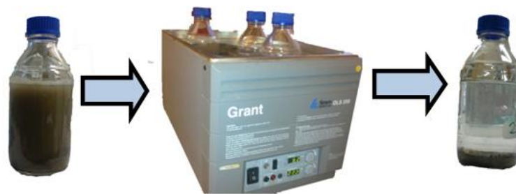
Figure 4.6: Batch Leaching process steps and equipment.
