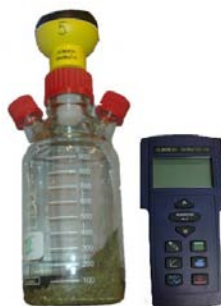
Figure 4.4 Photo of one of the OxiTop bottles complete of measuring head and controller used in the laboratory.
