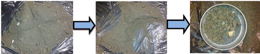
Figure 4.3: Sample preparation steps: quartering procedure and sieving.
