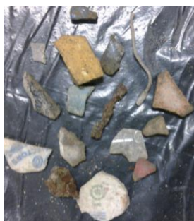
Figure. 1.2. Photo of coarse refractory material found after quartering and sieving in a sample of MSWI bottom ash. Is possible to recognize some pieces of ceramics, metallic material and construction-demolition waste.
