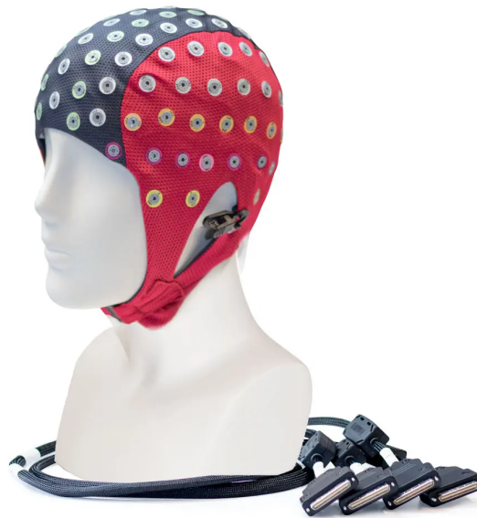
Figure 2.3: EEG cap: ANT Neuro EEG cap used for the EEG acquisition.
