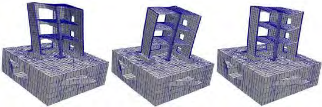
Figure 13: complete model modes 1 (6,23 Hz), 2 (10,28 Hz) and 3 (18,76 Hz)
