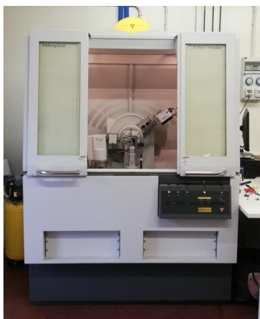
Figure 2.11 XRD analysis instrumentation
