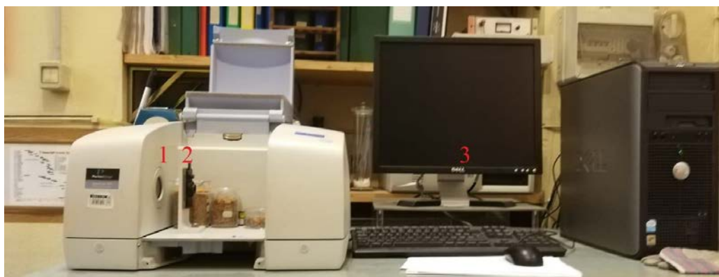
Figure 2.12 Instrumentation for the FT-IR Analysis
