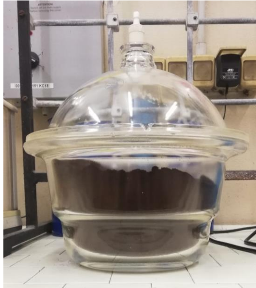
Figure 2.1 Desiccator containing the spent coffee grounds
