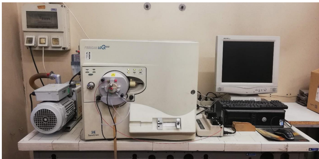
Figure 2.17 Instrumentation for the electrospray ionization analysis
