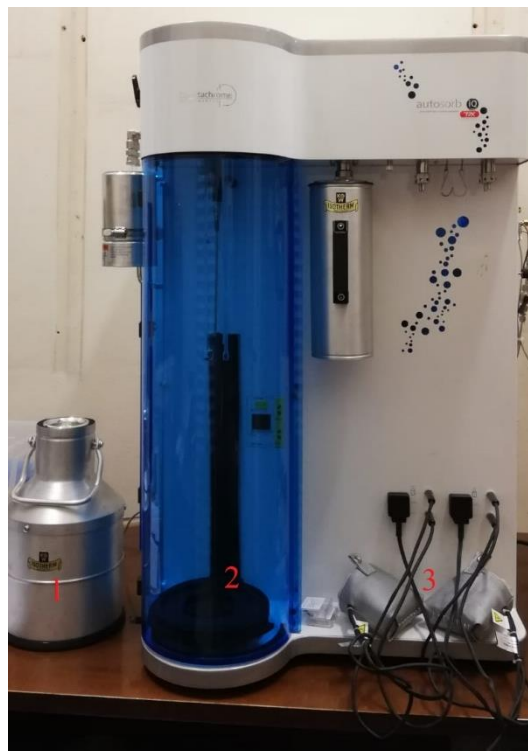
Figure 2.10 Instrumentation for the BET Analysis
