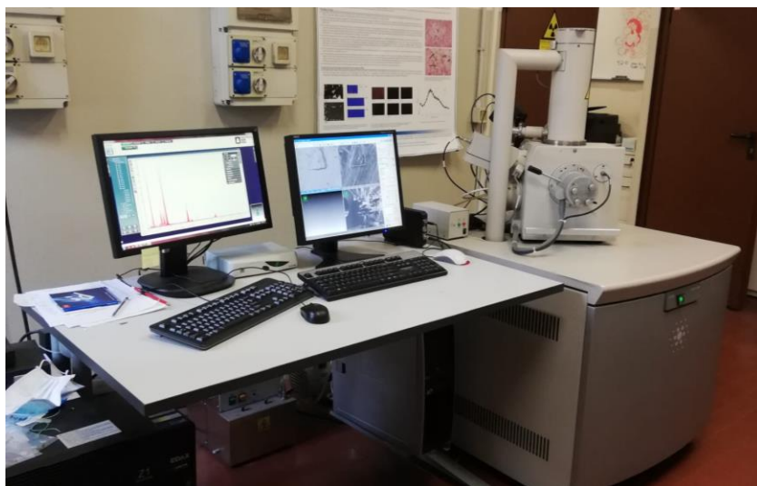
Figure 2.8 Equipment for the ESEM analysis
