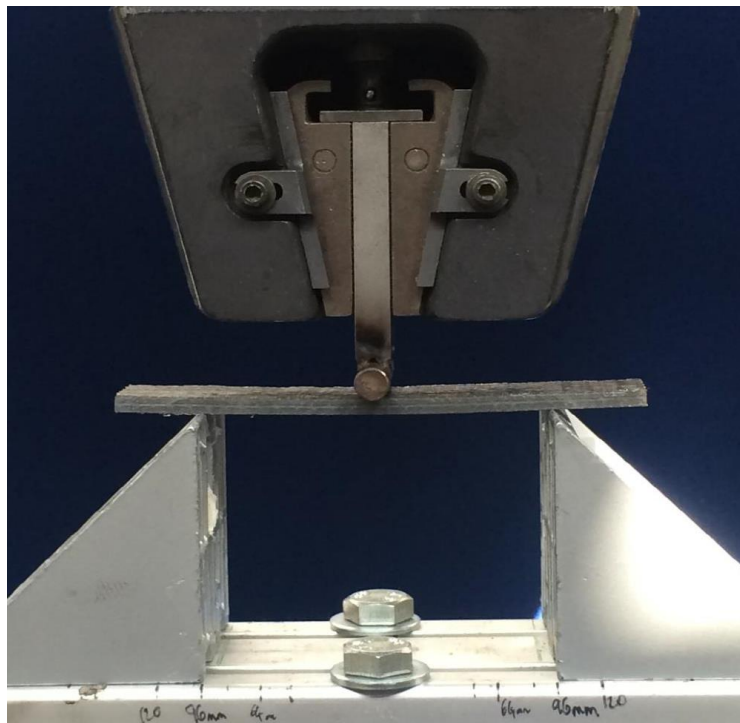
Figure 23. Three-point bending test apparatus
