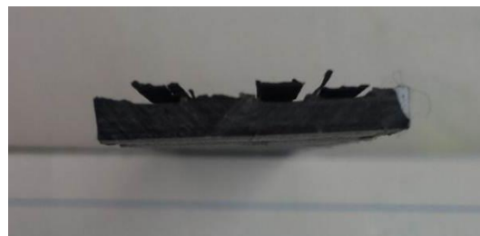
Figure 61: Specimen 1, delamination visible.
