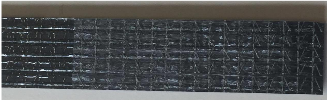
Figure 33: The interface at which failure occurred in a specimen with no interlayer.
