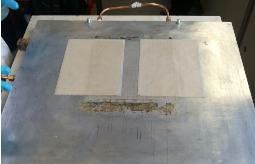
Figure 16. PTFE and release ply on the aluminium mold
