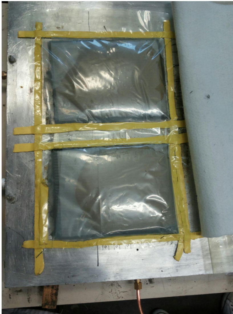
Figure 19. Inner bag with sealant tape (yellow). Breather visible on the right
