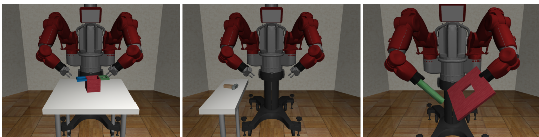
Figure 1.5: Baxter robot simulated into different Robosuite environments.
