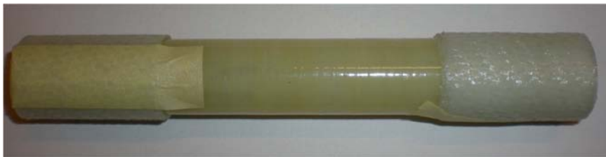
n) Specimen before tabs curing.
