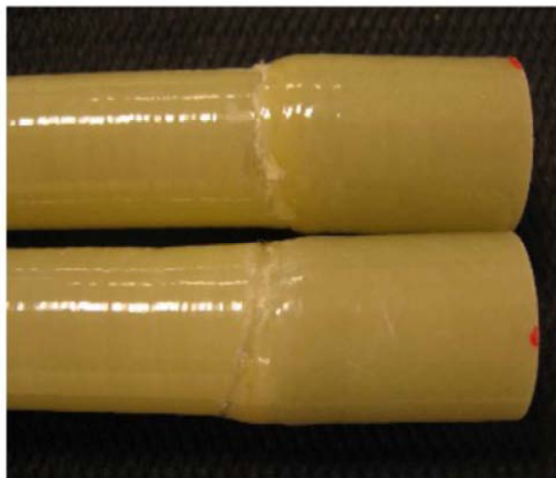
Figure 3.5 – Defects in specimens with integrated tabs (taken from [5]).
