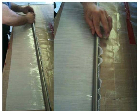
d) Attaching pre-pregs to mandrel.
