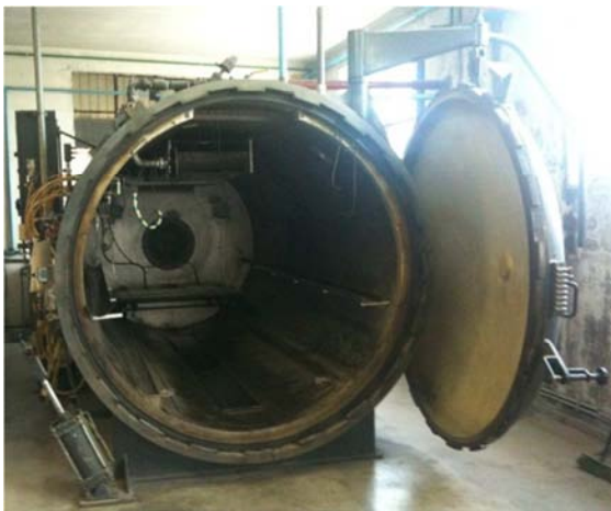
i) Autoclave used for curing cycle.
