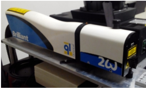
(a) Laser Brilliant Q-switched Nd:YAG .
