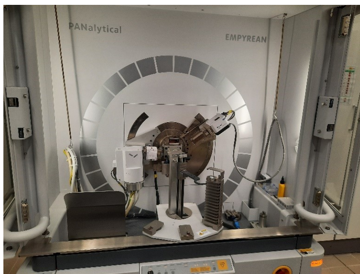
Figure 3.4: PANalytical Empyrean XRD Diffractometer SEGAI Labs at ULL used for the XRD characterization of the samples. The radiation used for the experiment was the Cu K- \alpha (1.54 Å) wavelength.
