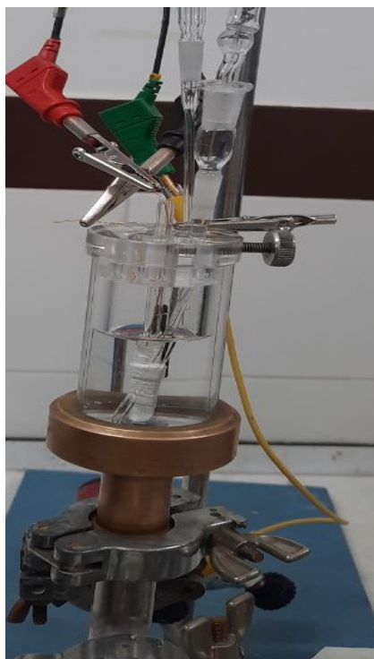
Figure 4.5: The electrochemical cell used in the DEMS system (a) with the glassy carbon rod used as CE, the RHE used as RE inserted in the Luggins tube, and the Teflon-wrapped glassy carbon rod touching the WE carbon cloth placed right on top of the Goretex membrane and the steel frit above the connection to the vacuum chamber.
