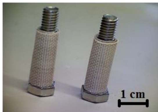
Figure 5.15: Bolts covered with a Teflon layer, employed for preventing the shrinkage of the clamping holes during the heating process.
