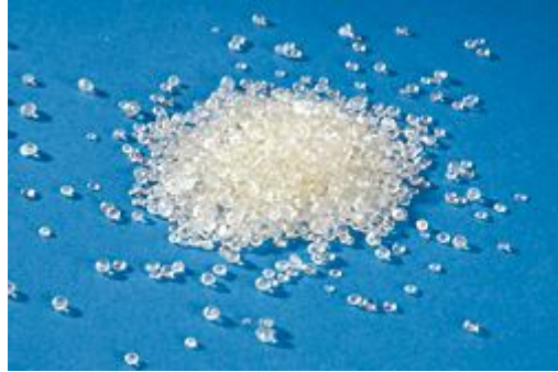
Figure 5.3: Pellets of phenoxy resin (PKHB) [36].
