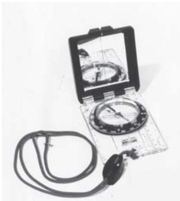
Figure 41: example of Compass designed for the geologist. In particular it is visualized a Finnish Suunto compass, similar to the Swedish Silva Ranger 15 TDCL. (from Lisle et al., 2011).
