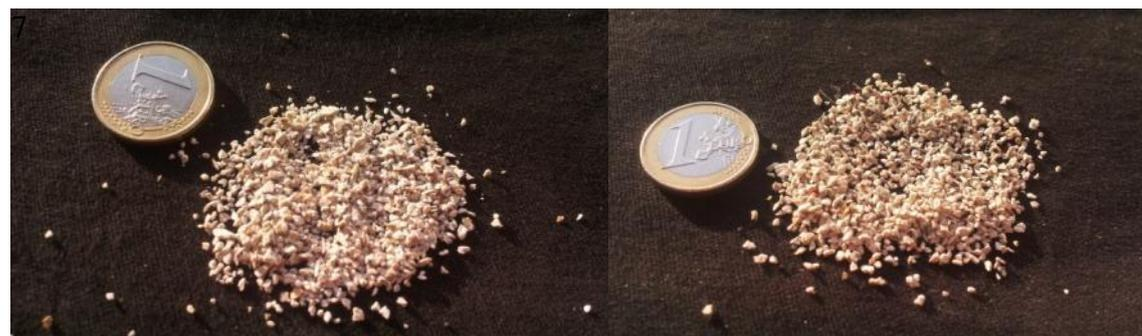
*Figure 73: Samples of Well AZ-35. On the left, 750 m depth sample (Dacite). On the right, 1050 m depth sample (Dacite). (CFE Petroteque at the Los Azufres Geothermal Field).*
