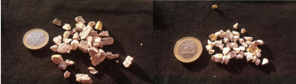
*Figure 71: Samples of Well AZ-35. On the left, 50 m depth sample (Rhyolite) . On the left, right m depth sample (Rhyolite). (CFE Petroteque at the Los Azufres Geothermal Field).*
