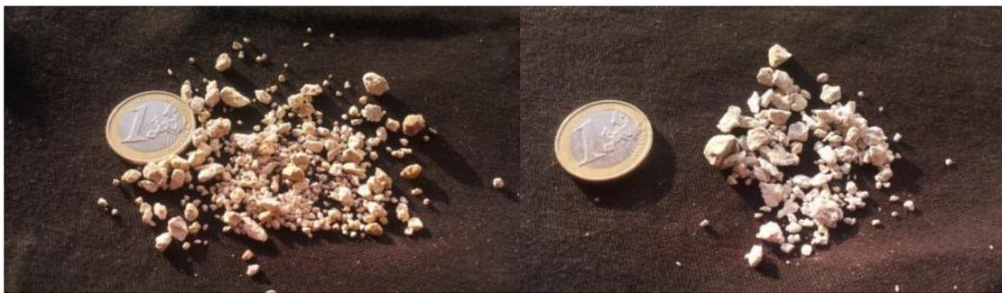
*Figure 72: Samples of Well AZ-35. On the left, 350 m depth sample (Rhyodacite). On the right, 500 m depth sample (Rhyodacitic tuff). (CFE Petroteque at the Los Azufres Geothermal Field).*
