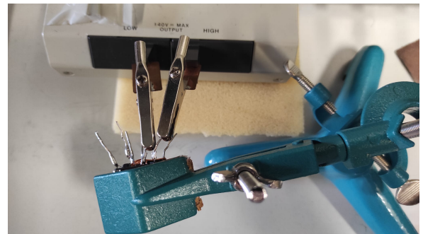
(b) Instrumentation set up: transformer connection.
