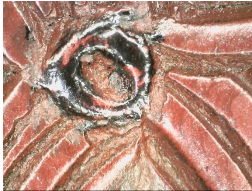
Figure 52 – Polychrome plate, spot (3). Black layer beneath red; middle black part shows incomplete abrasion.
