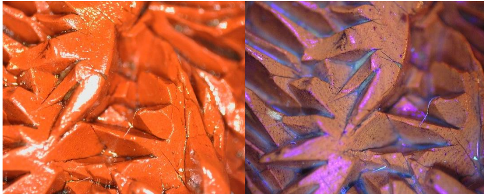
Figure 38 – Brush holder, spot (1). Left image: under normal lighting. Right image: under UV lighting.
