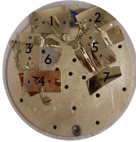
(a) Typical disposition of substrates during a sputtering run. In sequence, 5 nm of Ti, 45 nm of Ag and 10 nm of Au were deposited.
