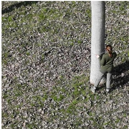
*Figure 3.14 Tree diameter measurements using caliper*
