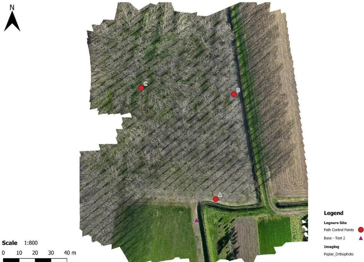
Figure 3.21 Control points during Field Survey 2, with new GNSS base position
