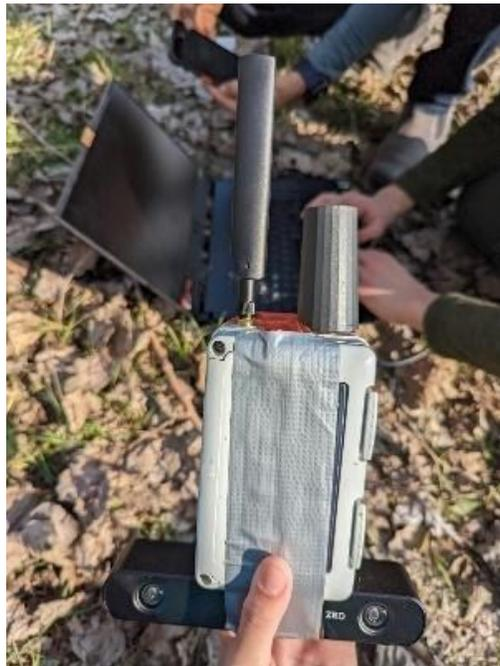
*Figure 3.15 Stereo Camera with rover centrally mounted on top*
