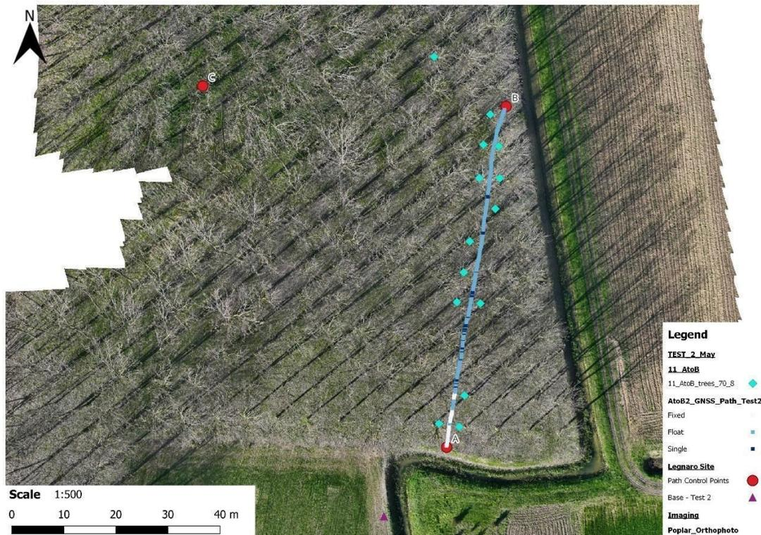
Figure 4.12 Test 2 path A to B consolidated tree positions with filtering of 70% confidence and 8m distance range
