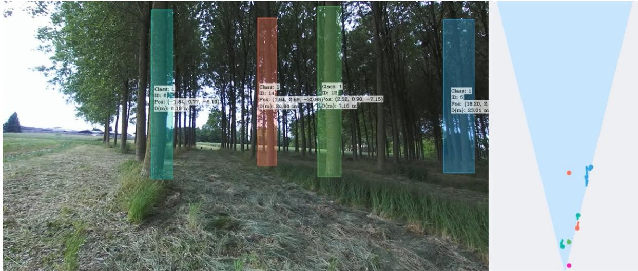
Figure 2.2 Sample video output screenshot from the ZED 2i Stereo Camera, showing real-time object identification (left) and 3D object tracking (right)
