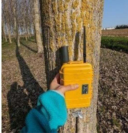
*Figure 3.13 Tree position control survey using Emlid Reach M2 rover*
