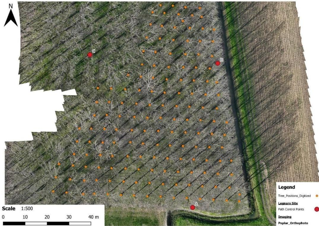
Figure 4.2 Legnaro site tree positions extracted from drone point cloud
