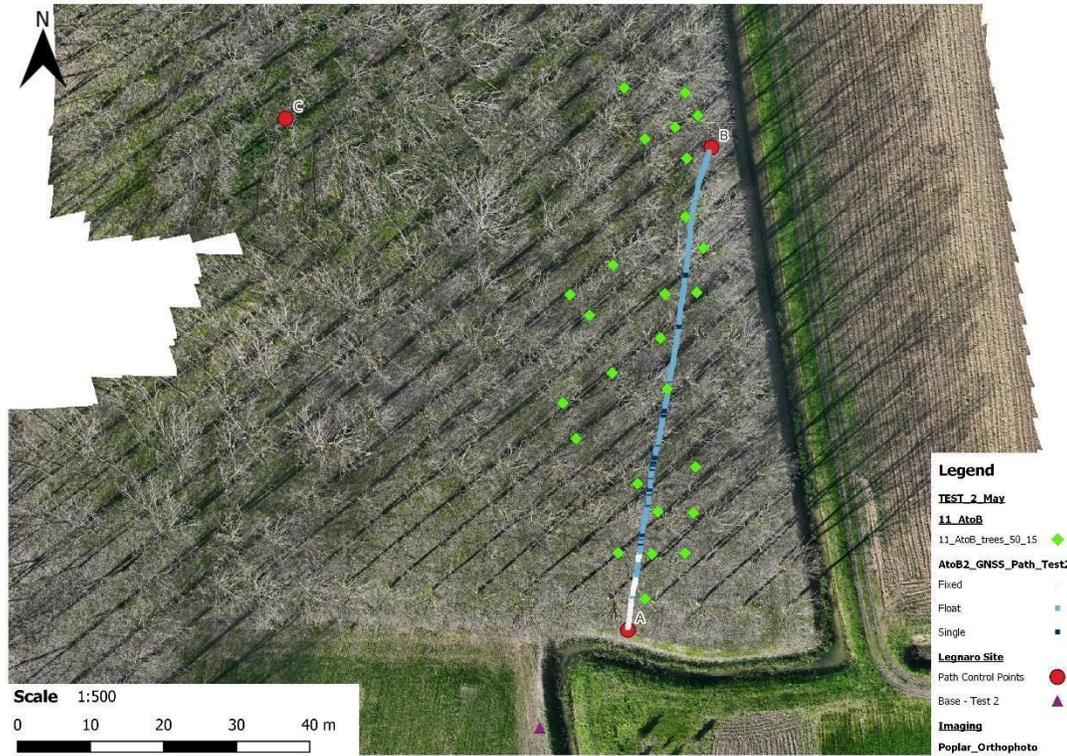
Figure 4.11 Test 2 path A to B consolidated tree positions with filtering of 50% confidence and 15m distance range
