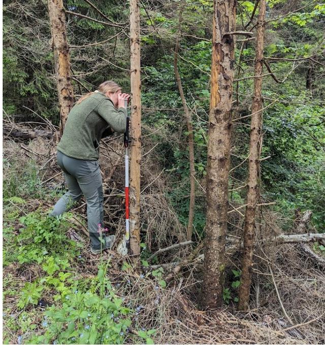
Figure 3.27 Use of Vertex Laser Geo to survey test area
