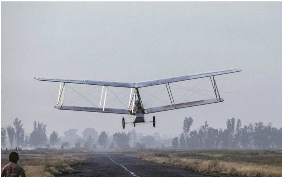
Figure 1.6: The Solar Riser was a improved version of the Easy Rider hang glider which combine aerodynamic facility with solar propulsion[18].
