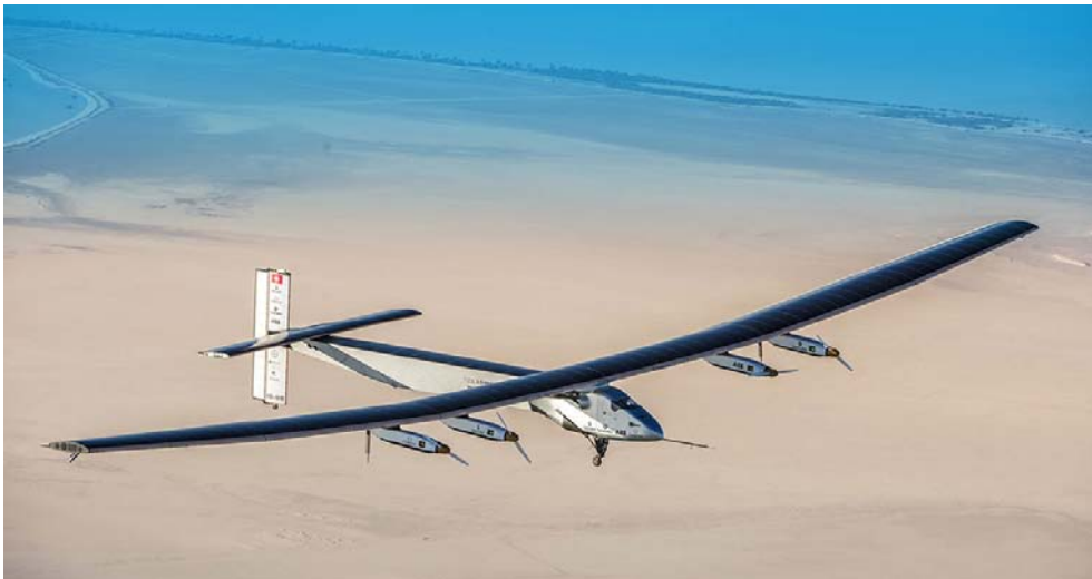
Figure 1.10: Solar Impulse 2 has a wingspan of 71 m, 22.4 m length, a cruise speed of 90 km/h during daytime and 60 km/h during night to save batteries. With it, Bertrand Piccard established new world record of circumnavigation in a solar airplane taking 16 months and 42000 km.[12].
