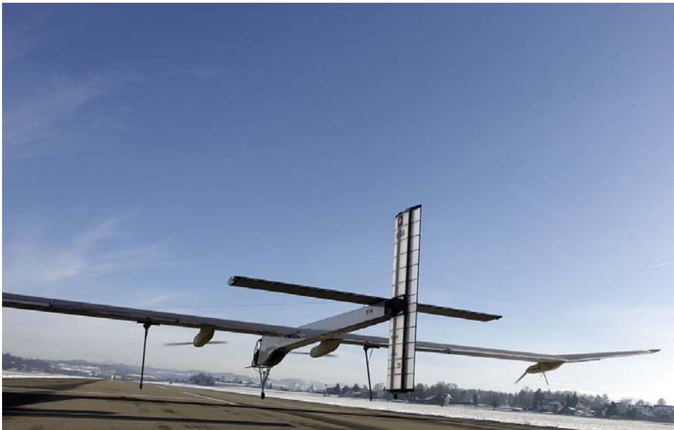
Figure 1.9: Solar Impulse 1, considered as a prototype for the successor Solar Impulse 2. Wingspan of 63 m, long 21.85 m and a take-off speed of 35 km/h. It weigh 2000 kg and has a cruise speed of 70 km/h. His funder and investor Bertand Piccard tested it flying from Switzerland to Spain and then to Marocco in 2010[12].
