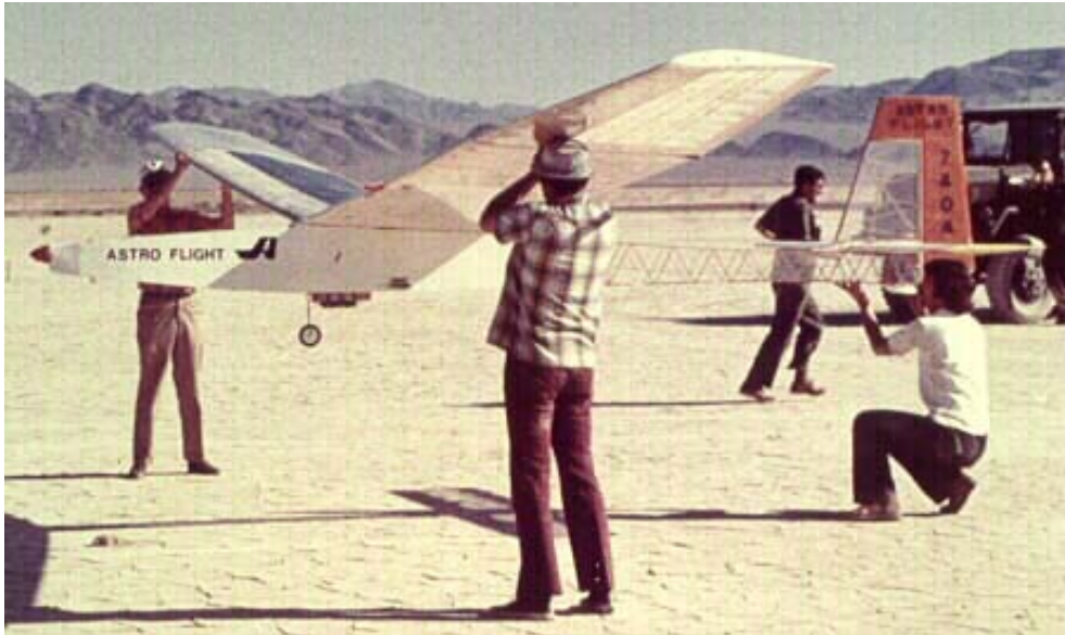
Figure 1.3: The first solar-electric powered fly machine, a model scale prototype developed thanks to Astro Flight Inc in collaboration with ARPA. It opens the way of solar powered aircraft future [18].
