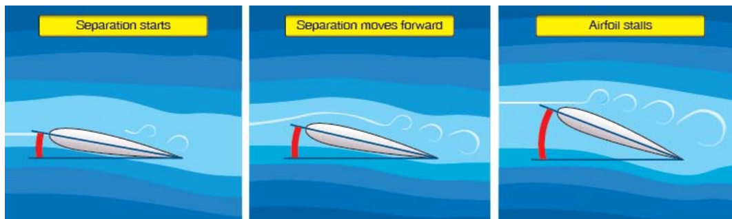
Figure 2.4: Three images of the same ideal profile at different angle of incidence[25].
