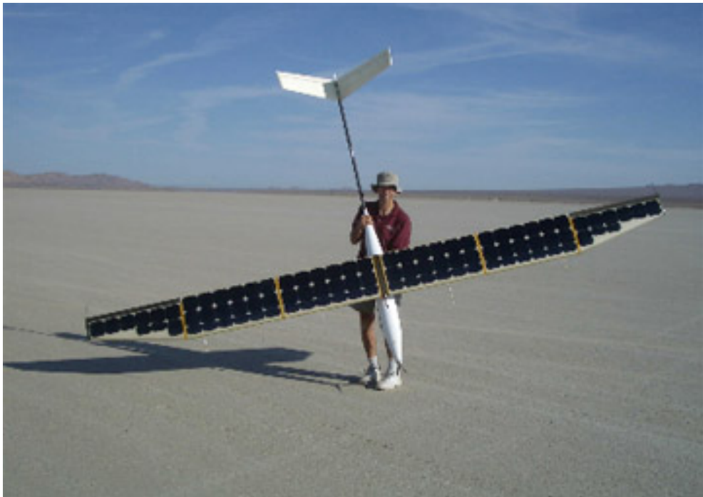
Figure 1.8: Little HALE model that break the barrier of 24 hours flight with only solar energy and batteries[18].
