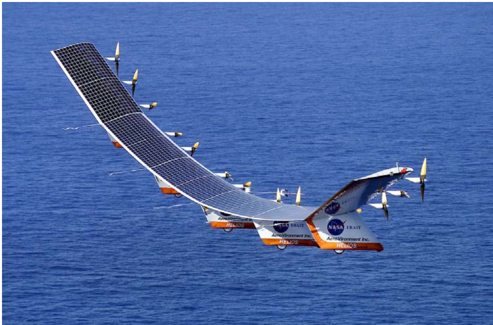
Figure 1.7: Helios project, designed to be the ultimate eternal plane and made by NASA. Improved from the previous project Centurion, it achieve the incredible altitude of 30 000 m (2001) before crashing on Pacific Ocean caused by structural fail in 2003[11].
