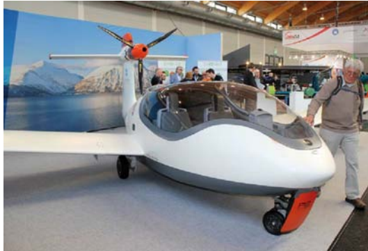
The Equator P2 , hybrid aircraft within the motor-generator Engiro G60 [1].
