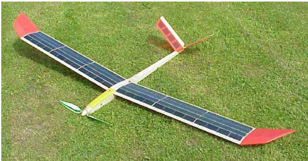
Figure 1.4: The solar powered model which held actual world records in longest rectilinear distance and duration [18].
