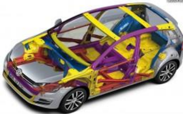
Figure 2. The body-in-white of the new Volkswagen Golf model year 2012 is more than 23 kg lighter than its predecessor, due in part to the intensive use of high- and ultra-high-strength steels; moreover it awarded 5-Star Euro-NCAP. (source: www.volkswagen.de )
