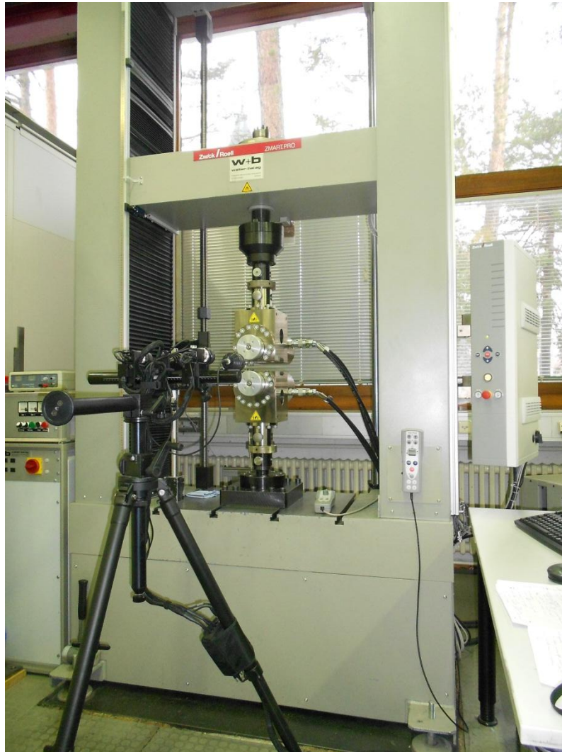
Figure 17. Tensile test machine Zwick/Roell ® ZMART.PRO and CCD camera.
