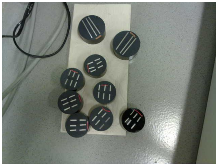
Figure 15. Embedments ready for metallographic analyses. The small ones are for heated and cooled side, the big ones are for the transition zone.
