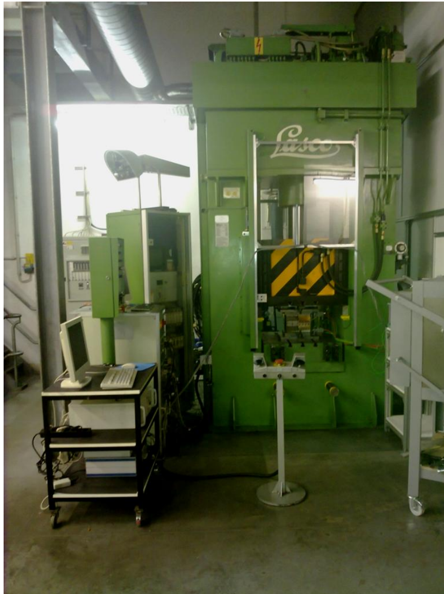
Figure 12. Facilities used during the press-hardening tests. Close-up, the Lasco ® press is visible; the furnace is on the right side of the picture.
