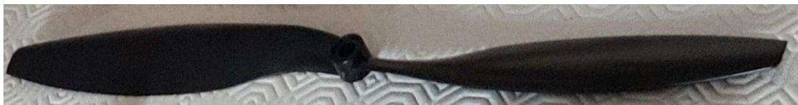
Figure 5.7 Elica 12x4.5 in materiale plastico
