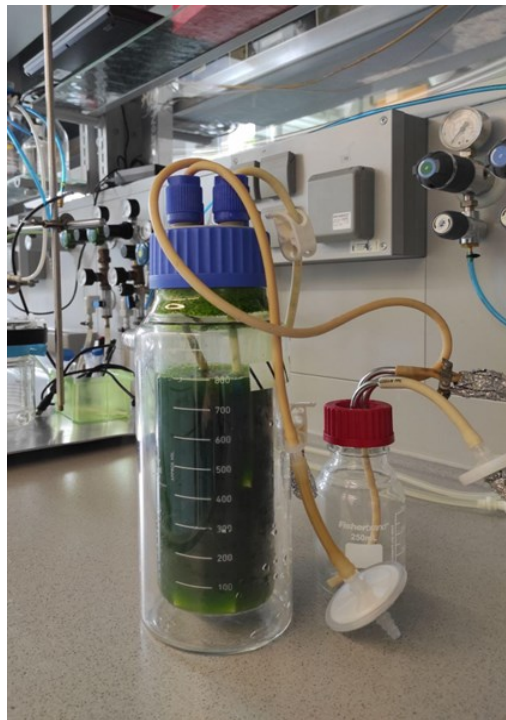
Fig 2.2 Bubble column PBR employed as pre-culture system at the University of Dresden (DWK Life Sciences GmbH, Germany)
