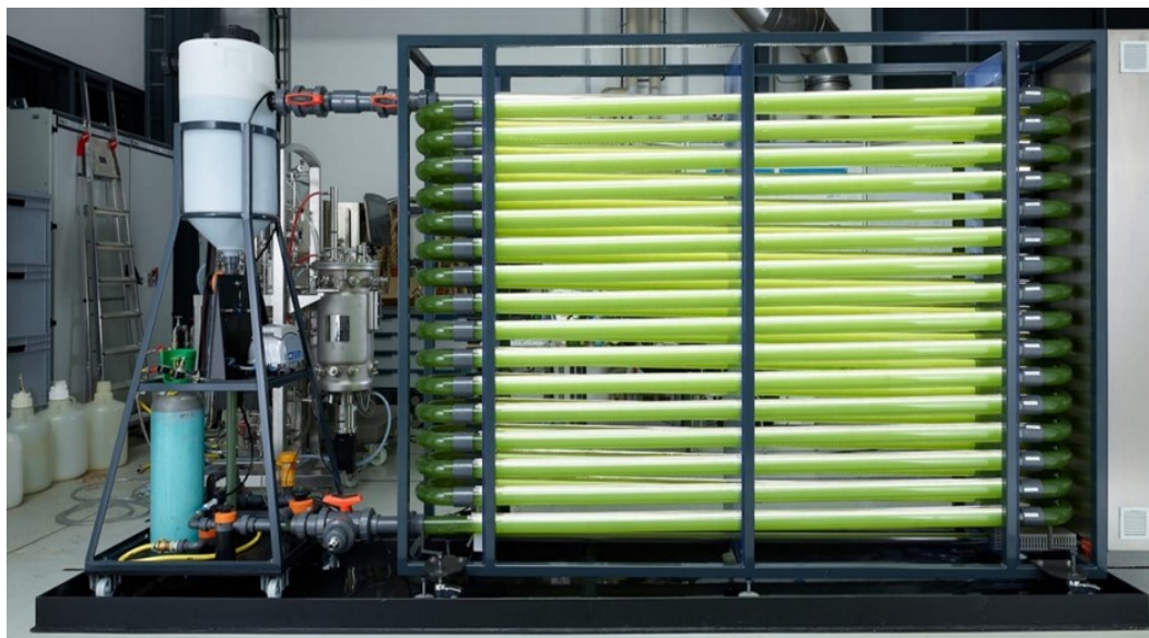
Fig. 2.3 200 L tubular PBR located at the university of Dresden designed by PUEVIT (PUEVIT GmbH, Dresden, Germany)
