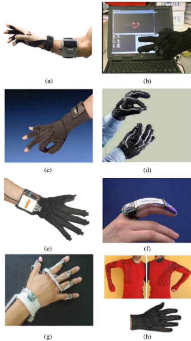
Fig. 2. Glove systems. (a) CyberGlove II. Reproduced by permission of Immersion Corporation. Copyright © 2008 Immersion Corporation. All rights reserved. (b) Humanglove. Image courtesy Humanware. (c) 5DT Data Glove. Image courtesy www.5dt.com. (d) Pinch Glove. Image courtesy Fakespace Systems. (e) Didjiglove. Image courtesy John Timlin, Didjiglove Pty. Ltd., Melbourne, Australia. (f) Fingemail Sensor [186]. Image courtesy H. H. Asada. (g) AcceleGlove [15]. Copyright © ACM. Reprinted by permission. (h) Upper limb garment prototype [187] and sensing glove [188] by Pisa University: sensors are directly integrated in Lycra fabrics by using conductive elastometers sensors. © 2006 IEEE and © 2005 IEEE.
