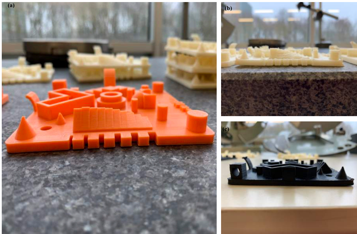
Fig. 4.21 – Pictures showing in detail benchmark part warping. (a) Prusa PLA high quality part, (b) Spiderbot ABS standard quality 75°C, (c) Prusa ABS high quality
