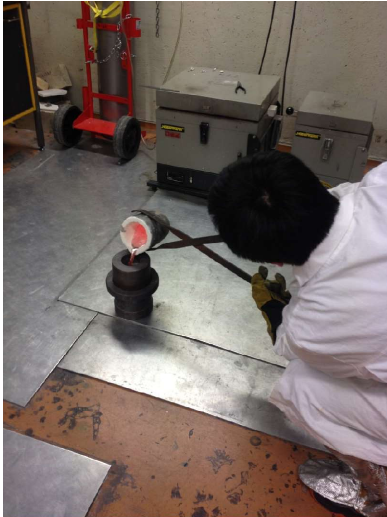
Figure 21 Pouring out of the remaining alloy in a Cu mould
