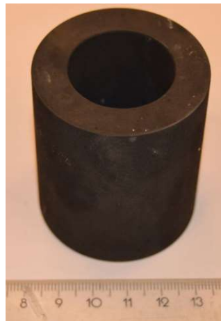
Figure 19 Small graphite crucible (scale bar in mm) used for the thermal analyses.
