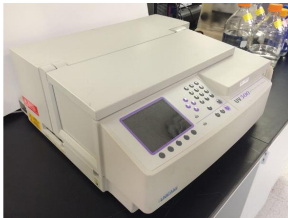
Figure 2.6 Spectrophotometer UV-500 UV-Visible (Spectronic Unicam). ( www.Labequip.com )
