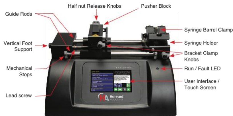
Figure 2.5 Harvard Apparatus PHD ULTRA™. (PHD ULTRA™ Syringe Pump Service User's Guide)
