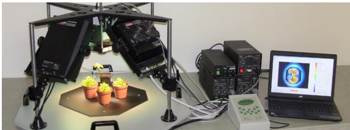
Figure 2.10 Open FluorCam FC 800-O (System Instrumentation). ( http://www.psi.cz/products/fluorcams/open-fc-800-o-1010 )
