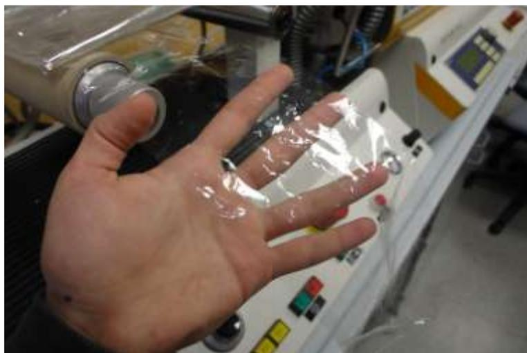
*fig. 6 – test filmatura in bolla PLA 4032D*
