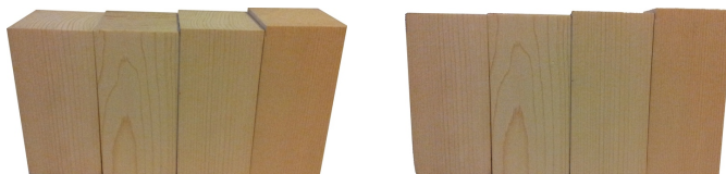
Figure 7.1: Test cubes used to measure the accuracy of our system; note the different heights of the four parallelepipeds.
