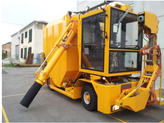
(b) Taphole breaking and covering vehicle.
