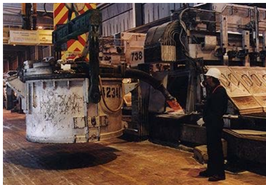
(a) Tapping operation by PTM with hanging ladle.
