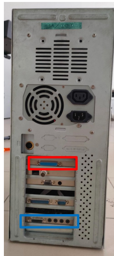
Figure 2.5: The Parallel Port (highlighted in the red rectangle) and the sound card (highlighted in the blue rectangle) of the original computer machine.
