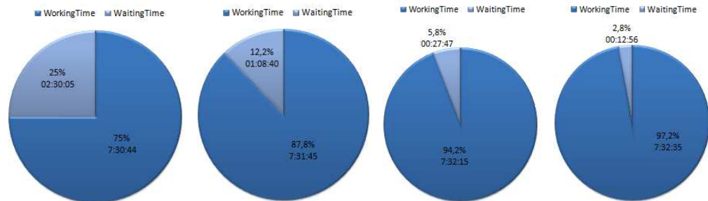
Chart 6.9 – Representation of the division of time in the Kiva system, with 3 batch orders and 3,4,5 and 6 robots
