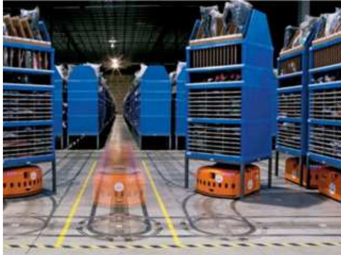
Fig. 2.8. - Navigation system of Kiva system (with fiducial markers)
