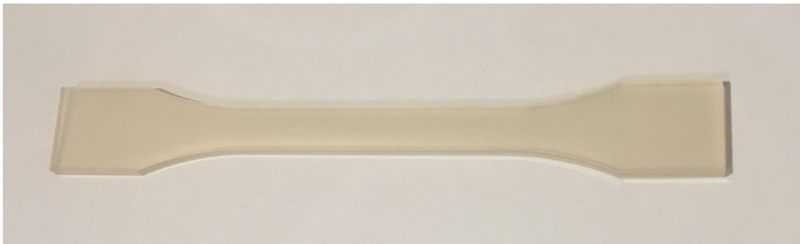
Figure 29 Mica45 3% dogbone specimen.
