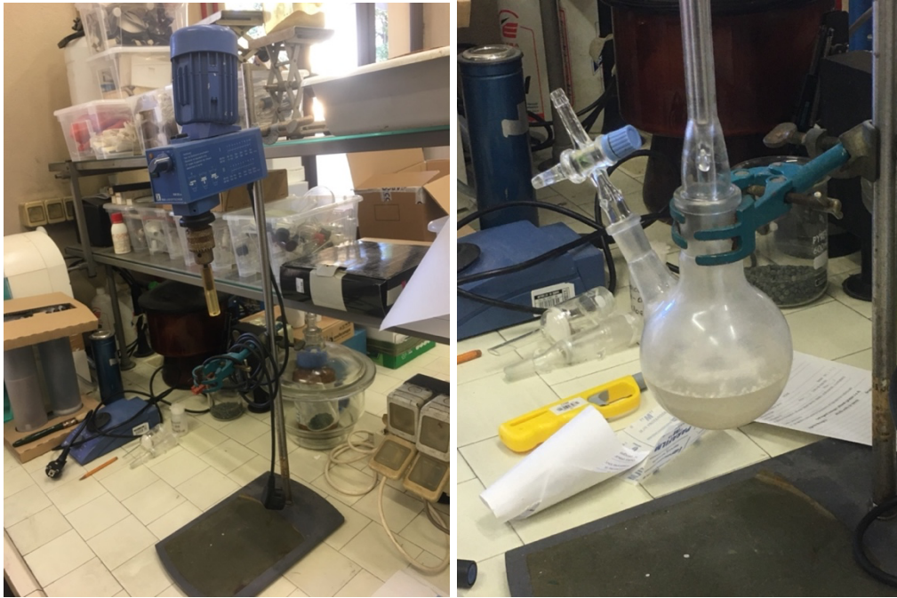
Figure 23 Photos from our laboratory. On the left, the mechanical mixer, on the right the mixing of the components during the specimens' preparation.
