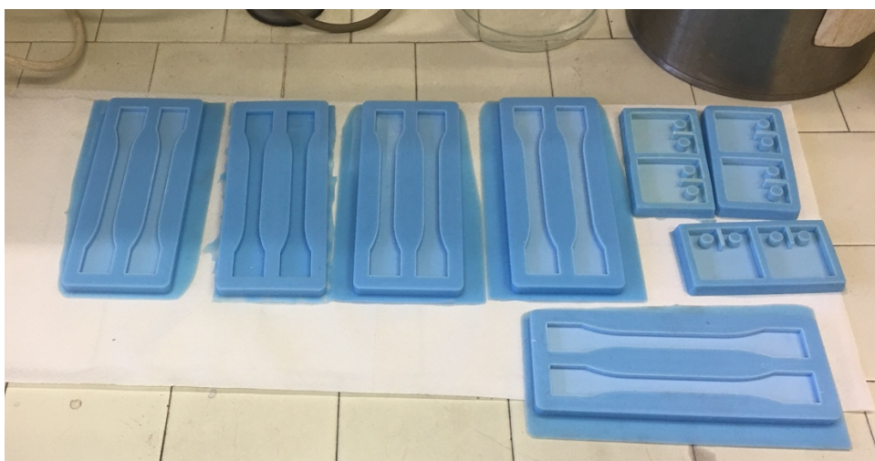
Figure 24 The silicone molds we employed in the specimens' preparation
