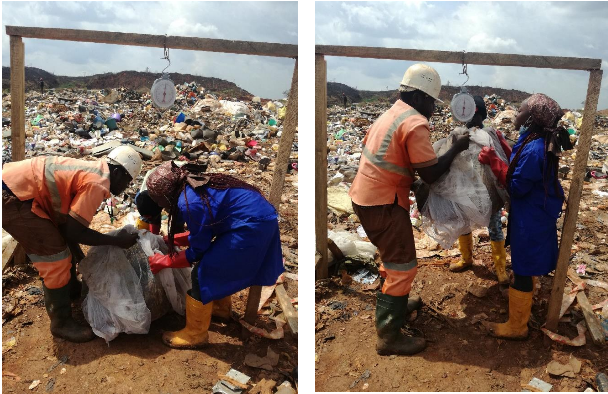
Fig 22: Readings from weighed waste (by category) on suspended scale
