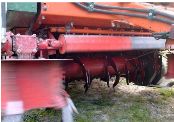
Figure 3a, b - Details of the vine-shoots harvesting unit used in the surveyed fixed-volume Gallignani round baler.
