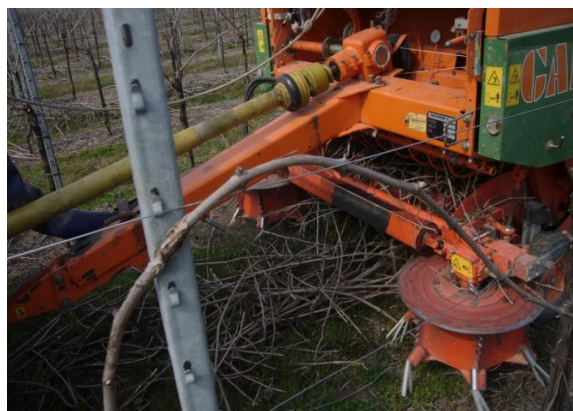
Figure 3a, b - Details of the vine-shoots harvesting unit used in the surveyed fixed-volume Gallignani round baler.
