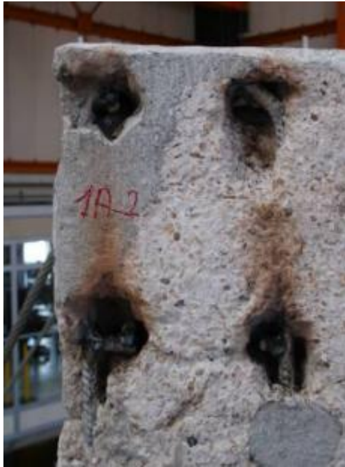
Figure 6.22: Welding the bars in Y-direction before test sequence 4 (Garcia et al. 2012)
