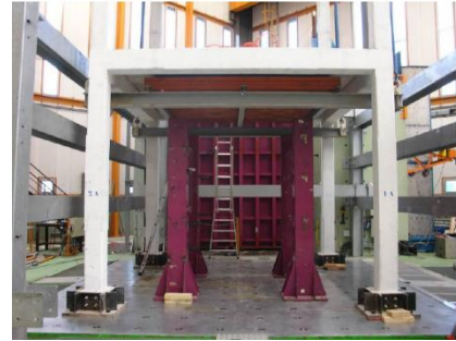
Figure 3.2: Clamping of the masses under first slab (Garcia et al. 2012)
