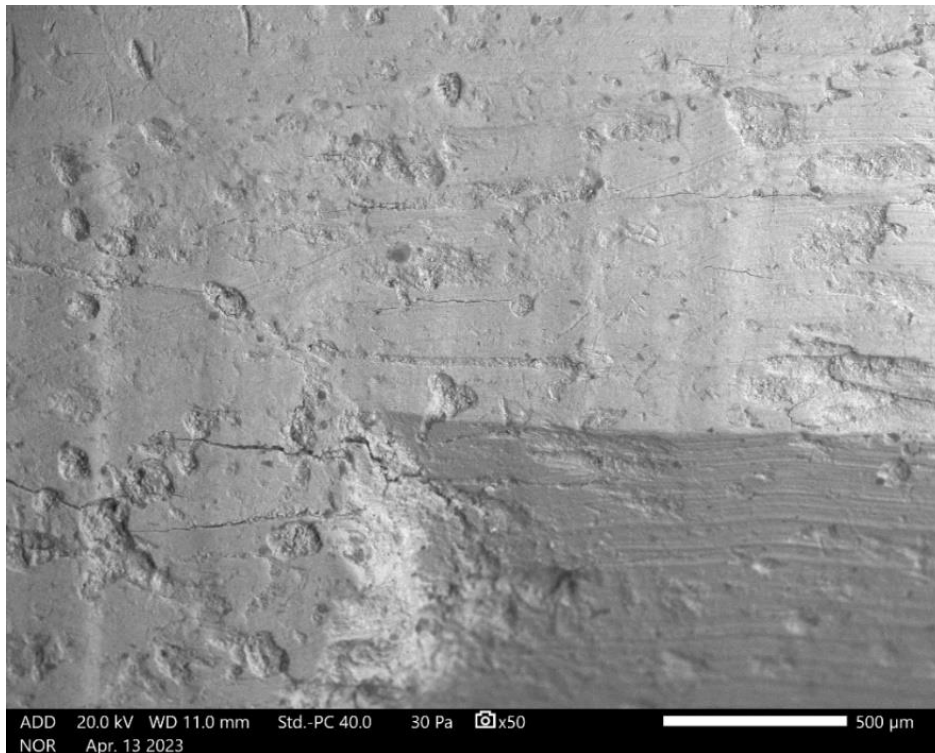
Fig. 81 - ESEM microphotograph of smoothing striations from the sample 3541.
