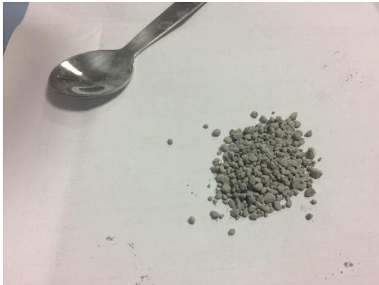
Figure 3.1. The coarser part of the slag A before it has been separated from the magnetic part and grinded.
