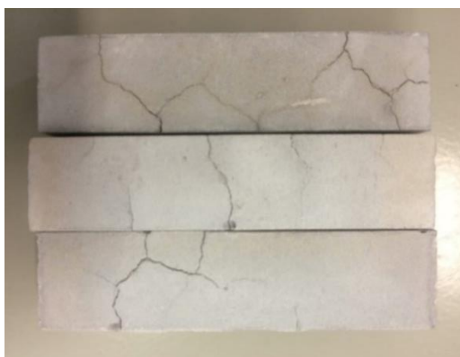
Figure 4.26. Fractures due to expansions in sample B5.
