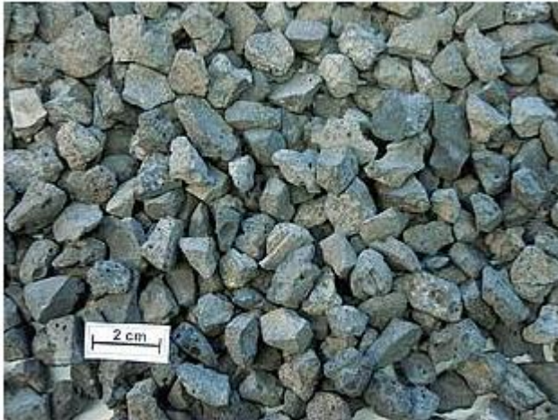
Figure 2.8. An example of Basic Oxygen Furnace slags (BOF), coarse aggregate (Euroslag, 2018).
