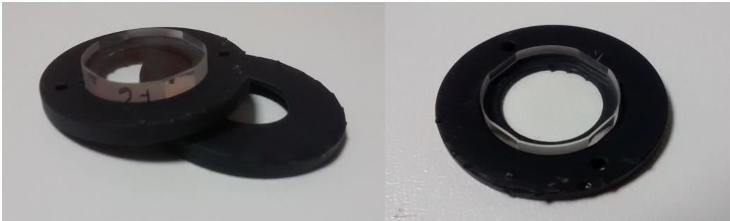
Figure 4.2: Images of the two pyramids: on the left the pyramid with divergent angle of 1^\circ ; on right the pyramid with divergent angle of 0.5^\circ . The vertex angles are so small that we can not notice in the images.
