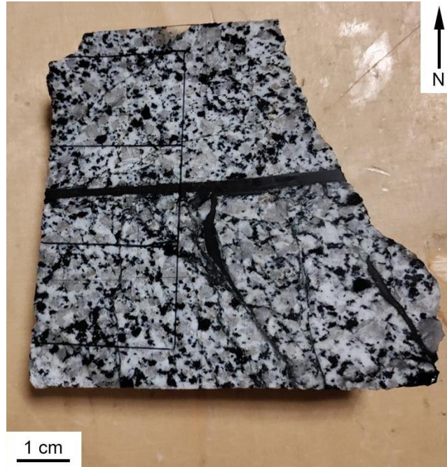
Fig. 3.2 Sample WF22-01 with location of the three thin sections: from N to S WF22-01a, WF22-01b, WF22-01c. WF22-01a and c are from the wall rock, while WF22-01b contains the ~ 2 mm thick pseudotachylyte-fault vein. To the right of the thin sections is located an injection vein intruding the southern wall rock.
