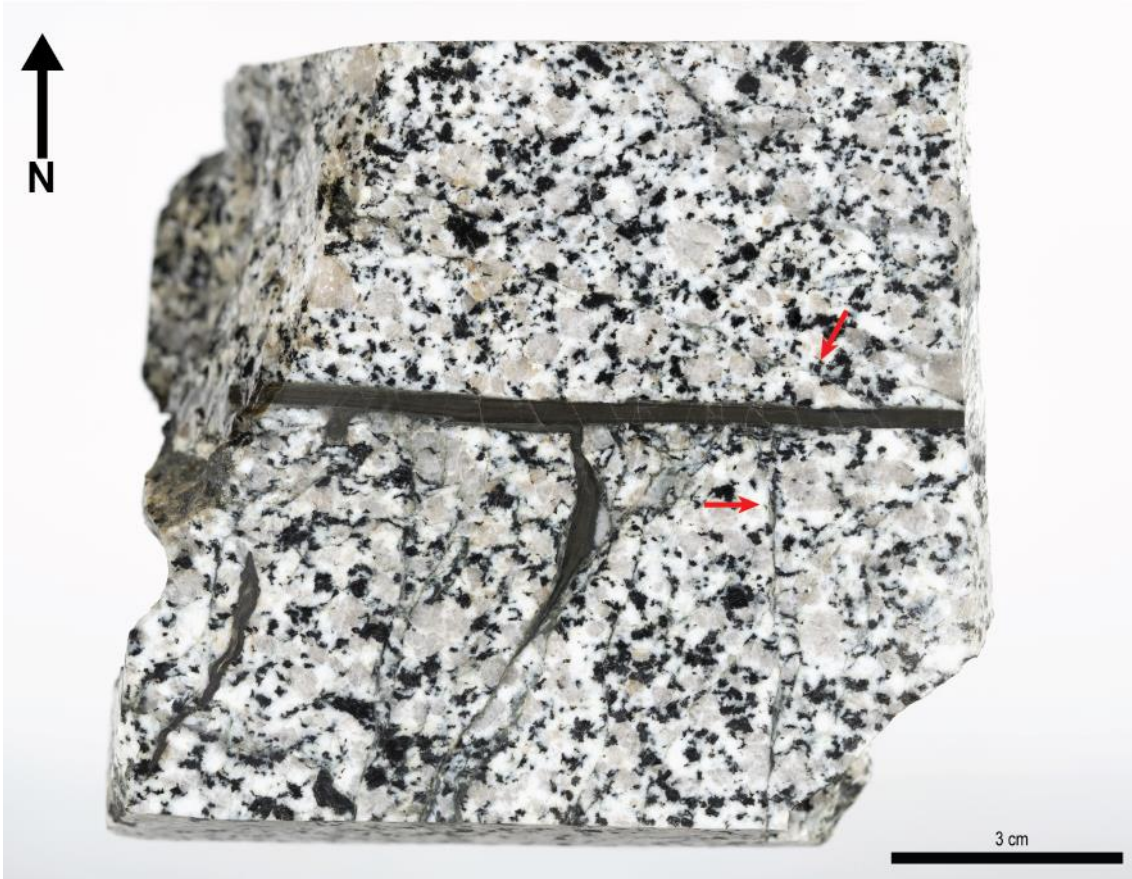
Fig. 4.3 High resolution photograph of the polished sample WF22-01. Red arrows indicate the fracture sets visible also in optical microscope micrographs of thin sections WF22-01a, b, c, to the right of a mesoscopic injection vein. (Fig. 4.9a, 4.10a).
