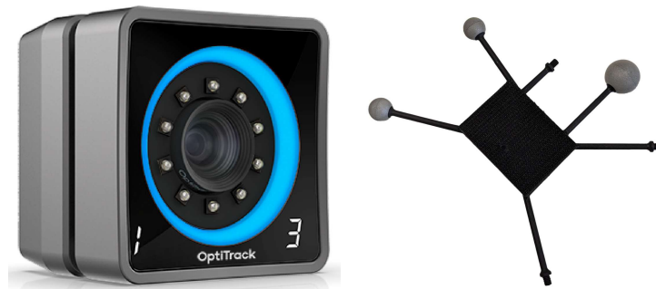
Figure 38: infrared cameras and infrared refractors used in the facility
