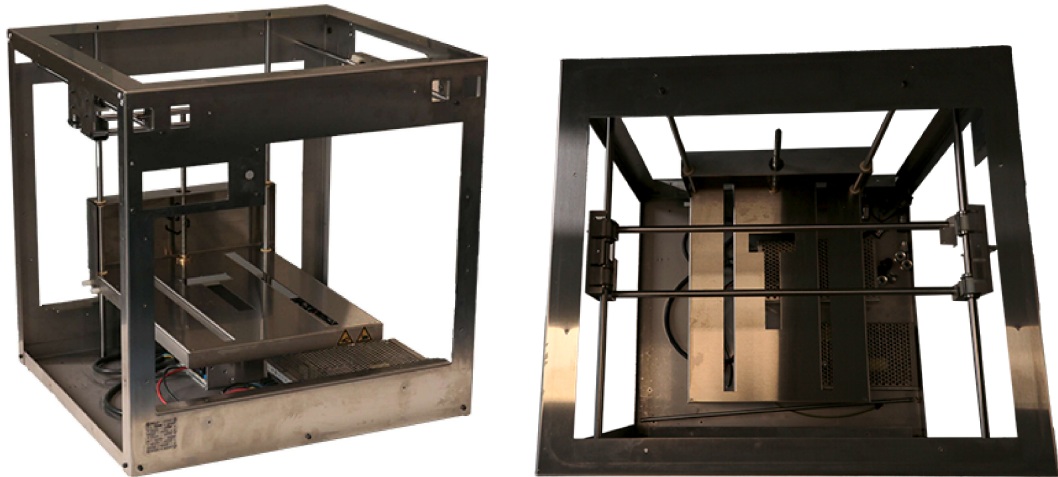
Figure 12: Kinematic test facility base structure with guides, side and top view
