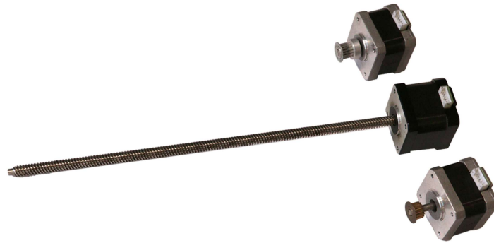
Figure 15: Stepper motors utilized in the kinematic test facility
