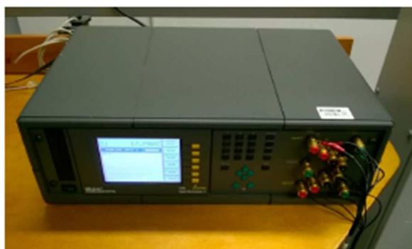
Fig. 14 Supertermometro (Hart Scientific 1590 1PPM Super Thermometer II)
