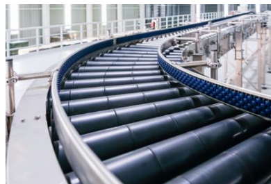
Figure 3.20: Example of a roller conveyor ( https://www.nai-group.com/conveyor-system-technology-trends/ )
