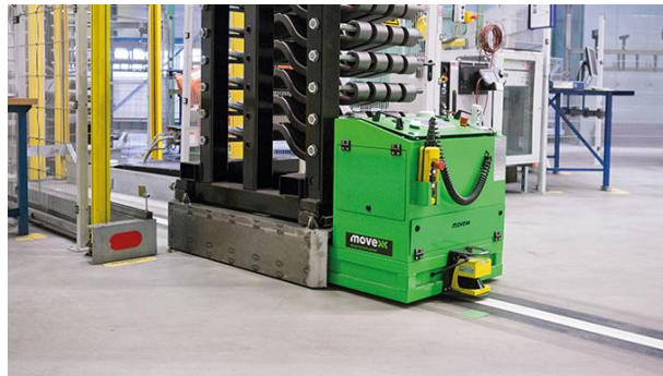
Figure 3.21: Example of fixed path AGV supported by photoelectric sensors ( https://www.turck.in/en/rfid-guides-agv-in-suspension-production-6880.php )
