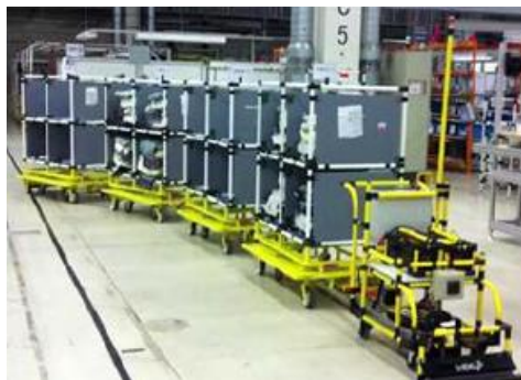
Figure 3.23: Multi load AGV (Battini et al. 2015)
