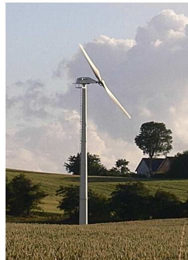
Figure 2: Gaia Wind turbine 11[kW]
