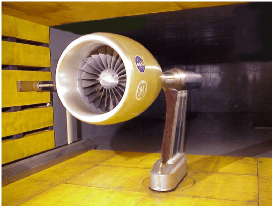
Figure 2.6: Fan module in the acoustic testing configuration installed on the UHB Drive Rig in the NASA Glenn 9- by 15-Foot Low Speed Wind Tunnel.
